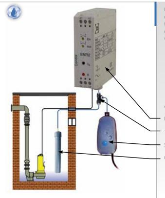
In this application, the aid of a small compressor is necessary, whereby in either continuous or periodic operation, air is fed into the system. The pressure within the measuring system (pneumatic tube) therefore remains constant. Only when a change in the level occurs is the pressure altered in the measuring system, which is subsequently detected by the evaluating unit.
