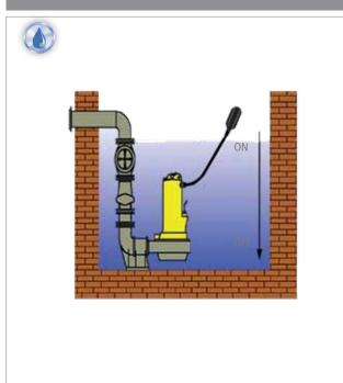
In this application, contacts placed within a floating enclosure are closed / opened depending on the inclination angle of the float switch.
