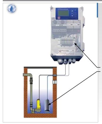
In this application, a level sensor is lowered into the medium within a sealed enclosure, whereby ceramic or piezoresistive sensors are used.
