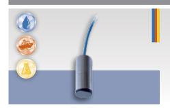
With ceramic measuring cell, shielded cable and a specially designed stainless steel enclosure, Condor offers a precision level sensor for all different types of applications, like e.g. wastewater. The sensor offers extremely high media resistance and the especially large membrane makes the sensor insensitive to pollution.
