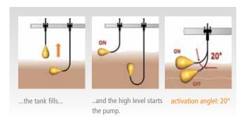
Used in couple with anoter of the same type allows you to adjust the levels of minimum and maximum. It's also possible to use a third and fourth regulator respectively for minimum and maximum alarm.
