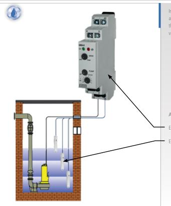
In this application, immersion electrodes are connected to an electronic analyser. When the electrodes are moistened by the liquid being measured, their conductivity alters corre-spondingly. One or two variable threshold values can then be adjusted.
