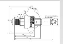
Pressure switch MDR 8 with EA + EV (on-off switch + unloaded valve)
