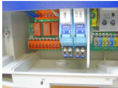
Fig. 2 Zener barriers in 2-pump operation - with divider -
