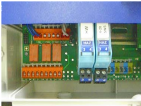
Fig. 2 Zener barriers in 1-pump operation - without divider -
