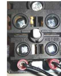
Counter wires connected to MOTOR/MOTOR terminal
